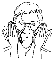
Figure 1 Negative Pressure Check
